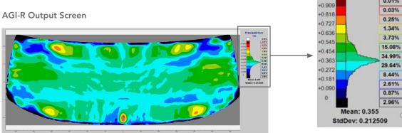
The AGI-R system has the capability to generate a simulated grid board or zebra board image. All parameters are user-defined including the viewing angle of the part. This allows users to see the effect of installation angle changes on the reflective optics by entering a new angle.
